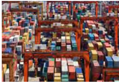
HIT is the first terminal operator in Hong Kong to deploy Electric Rubber Tyred Gantry Crane(eRTGCs)
