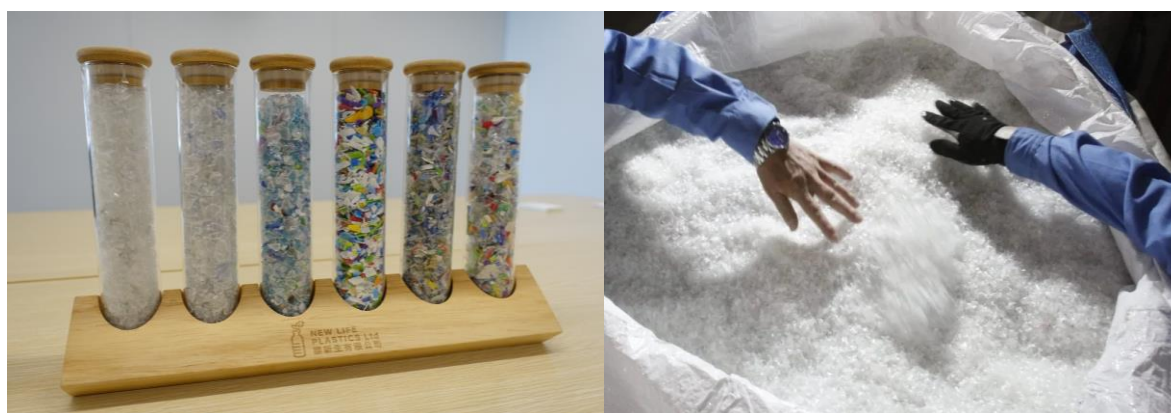
Figure 9: Left: Different grades of plastic recyclables separated by New Life Plastics Facility, with food-grade plastics having the highest value but hardest to derive due to stringent requirements and quality of incoming plastic waste stream. Other recycled plastics have wide application such as in the apparel industry. (Photo from site visit)
