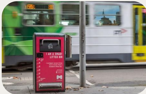
Figure 8. Smart bins that compact waste and hold seven times more than a standard bin have been tested in the innovation district of Melbourne 22
