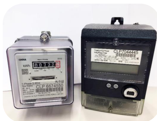
Figure 10. The Smart meter (right) with an associated communication system can collect near real-time electricity usage information 23
