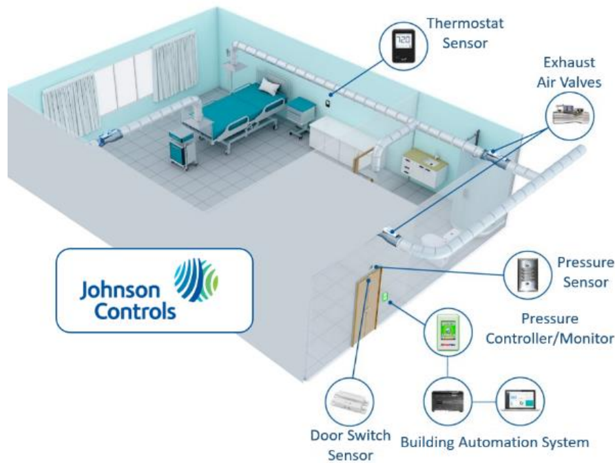
Figure 5. Smart HVAC solutions in a negative pressure patient isolation room (Johnson Controls) 10
